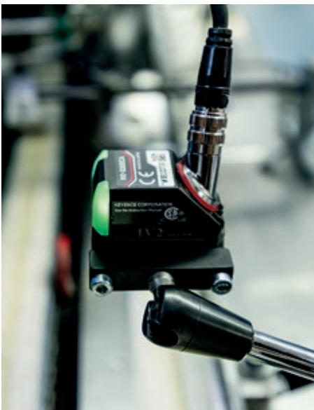
Specially developed camera system for perfect language allocation of letter and enclosure
