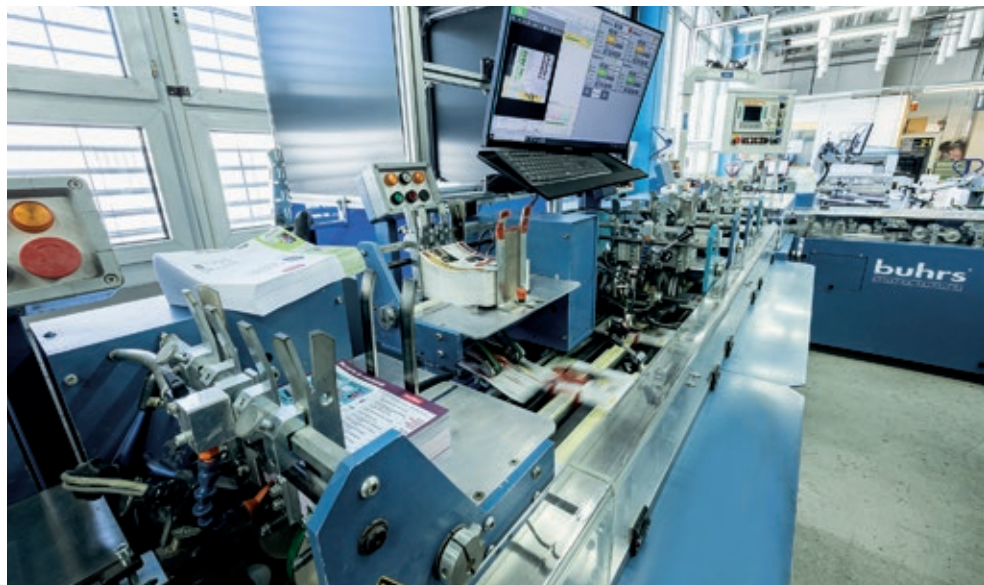
Specially developed camera system for perfect language allocation of letter and enclosure
